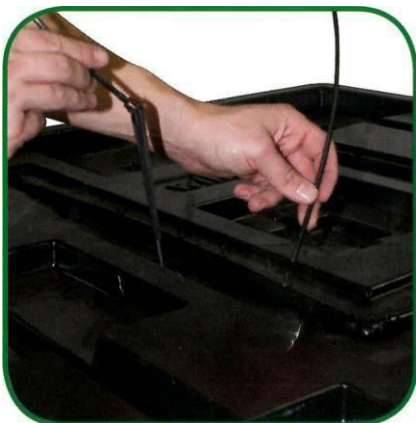
Fit Cobra hosing to nozzles
