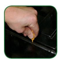
Pierce piping for fitting Cobra hosing in desired position
