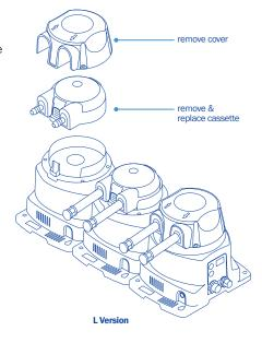
5 Replace the cover and screws, then reconnect dosing tubes.
