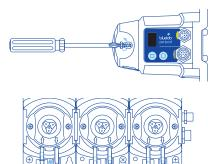
6 Connect power. Test pump operation, prime pump and tubes then calibrate the unit.
