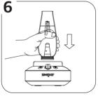
Carefully put glass cup on the vaporizer base
