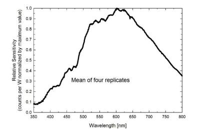
Sensitivity was determined by collecting spectra under a quartz halogen lamp with an NIST traceable calibration and calculating the ratio of counts measured with the spectrometer to energy flux density from the lamp. Maximum sensitivity of the SS-110 is near 600 nm. Sensitivity of the SS-110 is at least 10 % of the maximum value at all wavelengths greater than 380 nm.
