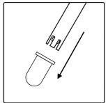
Immerse the tip (2.5 cm) of the EC probe into the sample. (for example it can float with the help of a piece of polystyrol).
