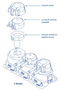
Replace the cover and screws, then reconnect dosing tubes.
