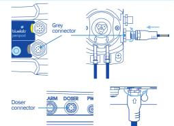
Line up connector pins, push and turn
