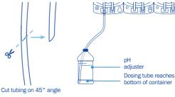
3 Set up the pH outlet dosing tube. M Version: use the remaining dosing tube with the connector, and insert the connector into the RIGHT pH pump tube.
