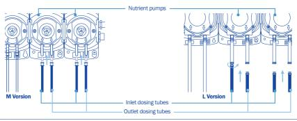
**Note:** If pH adjuster or nutrient stock solution being used has solid particles suspended in it, then a sieve filter should be placed on the end of the tube to prevent tube blockages and potential damage to the peristaltic pumps.
