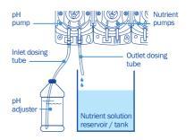
5 To set up nutrient tubing and pumps, repeat steps 1-4 using the darker nutrient solution tubing. For the L Version: Insert and twist each connector of the nutrient dosing tube into each nutrient pump tube connector.
