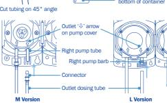
Out the outlet dosing tube so that the tube sits above the maximum solution level of the reservoir. The pH adjuster and nutrient solutions must drip into the nutrient reservoir.
