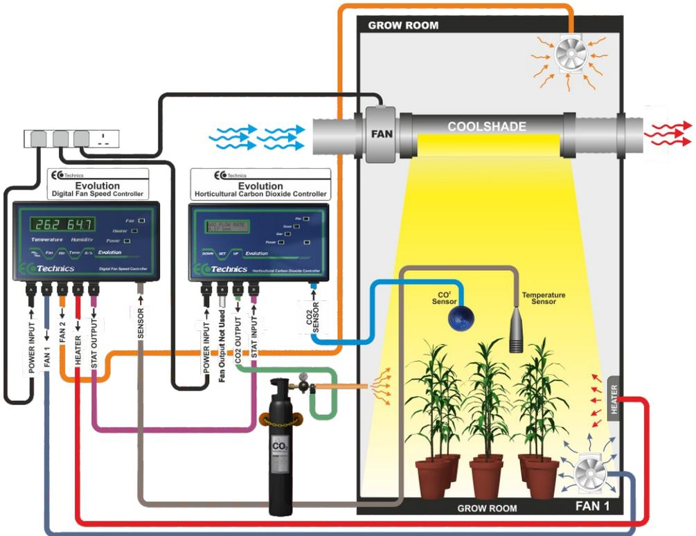
When the 2 Evolution controllers are connected together the fans should be connected to the Evolution Digital Fan Speed Controller as shown in the diagram above.
