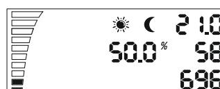
As the countdown ends without getting a light interrupt at the light sensor the controller will switch from night to day time or reverse from day to night time. Enter SET/SAVE to change the values.
