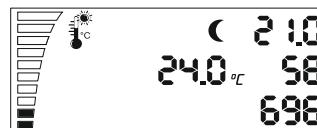
This last setting is the switch over time between day and night mode. This is used to avoid an immediate switching between day and night mode.
