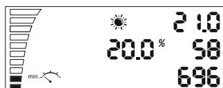
On the down left side speed bar you can see the actual setting for each filled segment is 10% fan speed. Change the settings again with SET/SAVE as described above.
