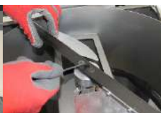
2 Loosen the central screw of the shaft.
