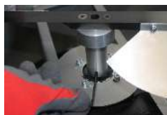
1 Loosen the lock screw shaft
