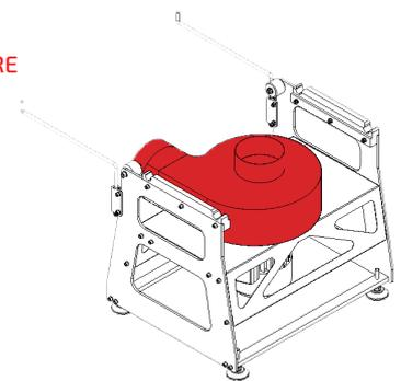
CLEAN WITH WATER UNDER PRESSURE AND MASTER CLEAN (D) FOR DISINFECTION.
