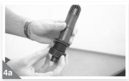
Remove the nut from the overflow fitting.
