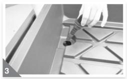
Connect the pump inlet fitting to the table by removing the nut and pushing the threaded end through one of the holes before securing in position with the nut.
