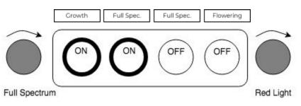
GC 16 plus comes with two *full spectrum modes* and two additional dimmers, controlling full spectrum and red light. The intention is to increase full spectrum during the grow period and to increase red light during flowering period without lowering the full spectrum.
