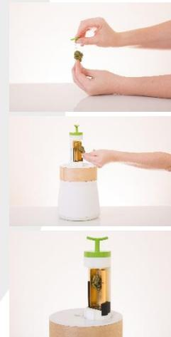
7. Stick flower pin into the flower and insert the pin into sample holder or alternatively stick flower onto the flower pin while it is within sample holder; whichever way you're comfortable with.
