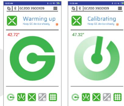
**Note:** Be fast - Analysis must commence within 1 minute of Calibration completion.
