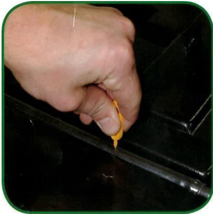
Pierce piping for fitting Cobra hosing in desired position
