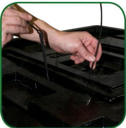
Pierce piping for fitting Cobra hosing in desired position
