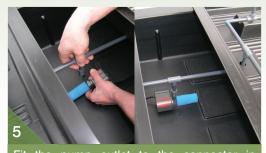
Fit the pump outlet to the connector in the middle of the T bar. It is a tight fit and may require some force. Attach the pump connector on each delivery system to each end of the T bar. You will probably need to lift both chamber bases slightly to put the pump into position. Secure it to the bottom of the nutrient tank with the rubber sucker.
