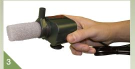
Fit the strainer and foam filter to the pump inlet. Make sure the pump outlet is at 90 degrees to the main body of the pump. Move the foot and sucker to the bottom of the pump so the pump outlet is upright.
