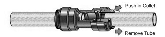
Push tube firmly into the fitting connector all the way to until the tube stops. Try to pull the tube out to check the security. If the tube pulls out, then push all the way in again.
