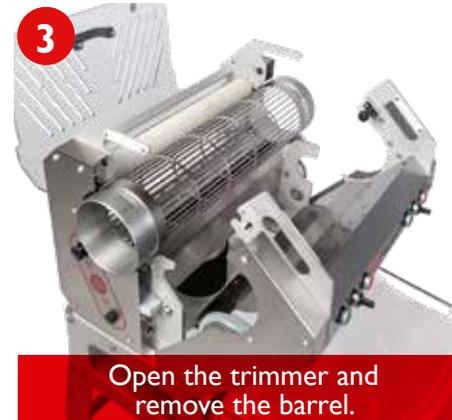
Open the trimmer and remove the barrel.
