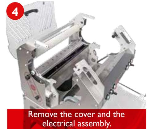
Remove the cover and the electrical assembly.
