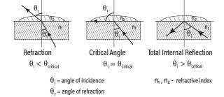
In the MA871, light from an LED passes through a prism in contact with the sample. An image sensor determines the critical angle at which the light is no longer refracted through the sample. The MA871 automatically applies temperature compensation to the measurement and converts the refractive index of the sample to sucrose concentration in units of percent (by weight) Brix.
